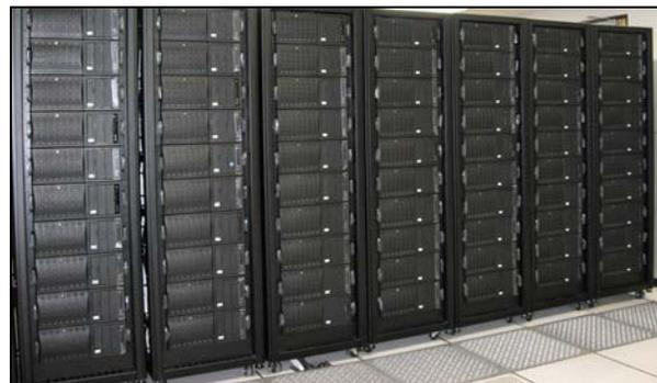
**Figure 1. Joshua cluster at J9 consisting of 256 dual quad core Opteron processors and 256 NVIDIA GTS8800 GPUs (Source: Ed Aaron, USJFCOM).**
