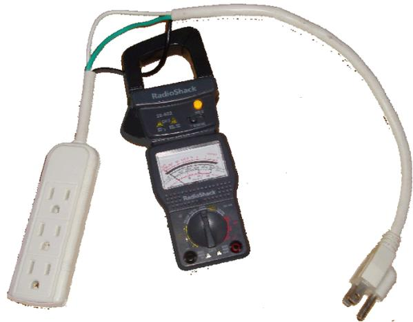
**Figure 3. Ammeter and harness used for current quantification**
