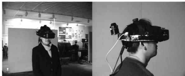
**Figure 8 – Head-mounted haptic display. (Now smaller)**
