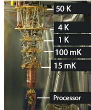
**Figure 6 - D-Wave Cooling Mechanism (D-Wave photo)**
