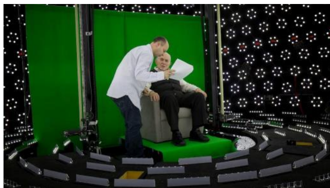
Figure 4 – Subject receiving direction in light stage used for generating 3-D imagery for holographic display
