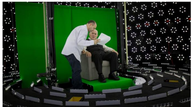
Figure 6. Subject receiving direction in light stage used for generating 3-D imagery for holographic display
