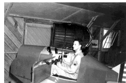
Figure 3 Link Flight Trainer, hood up
